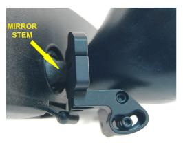
While sitting in the passenger seat, place the mount over the mirror stem. Tighten the CLAMP SCREW until the mount starts to clamp onto the mirror stem. Position the mount as far forward as it will go and paralell to the bottom of the mirror before fully tightening.
