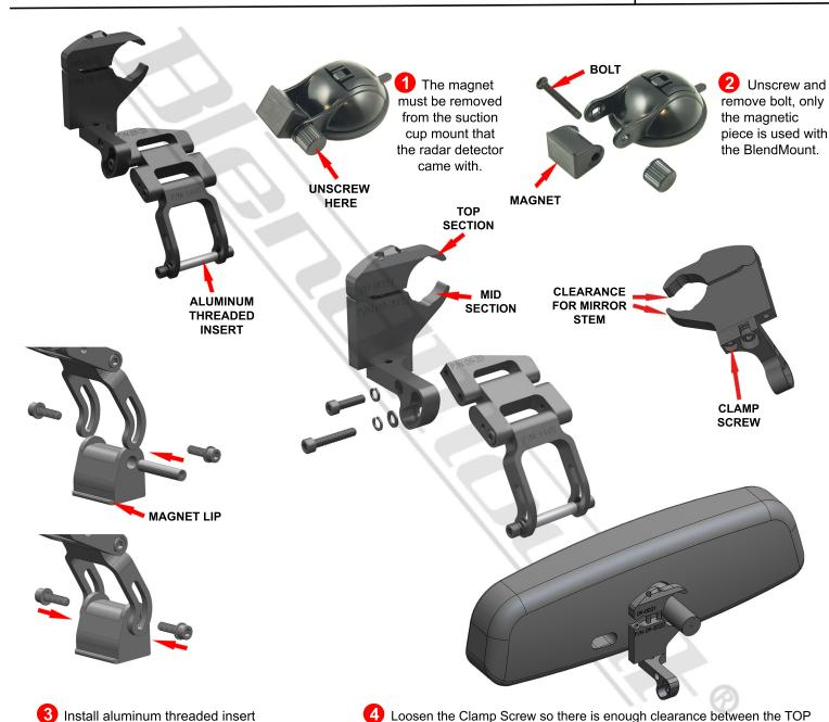
and MID SECTIONS to slide over the mirror stem. (P/N should be facing to-
